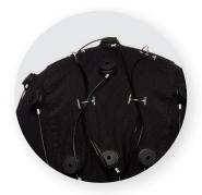
Sintered Ag/AgCl electrodes provide reliable signal quality overtime with no signal degradation.
